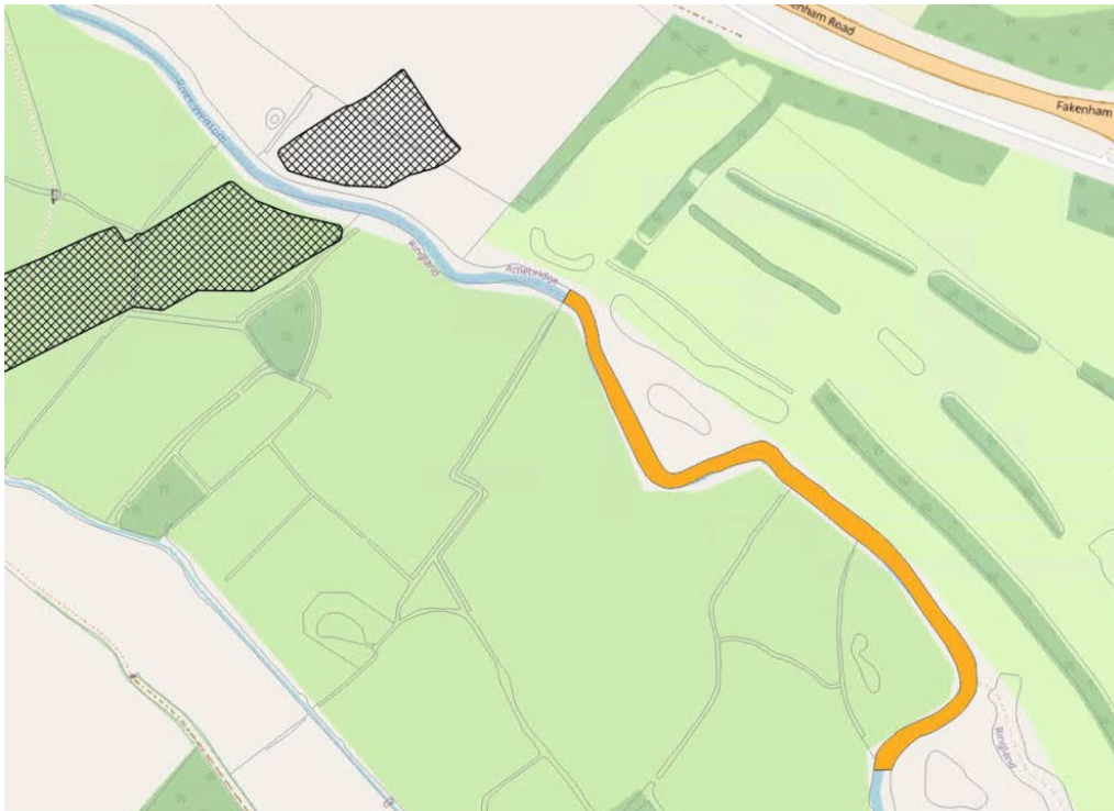
Figure 1.3 – Reach downstream of the proposed scheme. The hashed area corresponds to the temporary works platform required to construct the viaduct over the River Wensum
